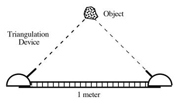
2. Stand a known (measured) distance from the chalk board. Measure the angle of a mark on the far wall of the lab room as viewed from each end of the meter stick.
