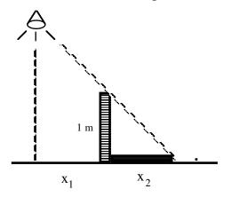
3. Calculate on the basis of similar triangles the height of the lamp.
