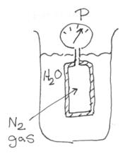
To measure temperature T of water using a constant volume gas thermometer, you immerse the small rigid gas tank in the
