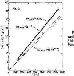
FIG. 1. Inverse magnetic susceptibility of  $Gd_2O_3$  as a function of temperature.
