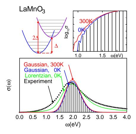
The spectrum is predicted to have the form of a "Franck-Condon series" of vibrational sidebands. In the absence of self-trapping, only the central band would appear. The experimental line-shape is broad, with only weak temperature dependence. The theory predicts that the low frequency wing of this broad line should show characteristic frequency-dependent and temperature dependent structure, illustrated in the log-scale version shown in the upper right.
