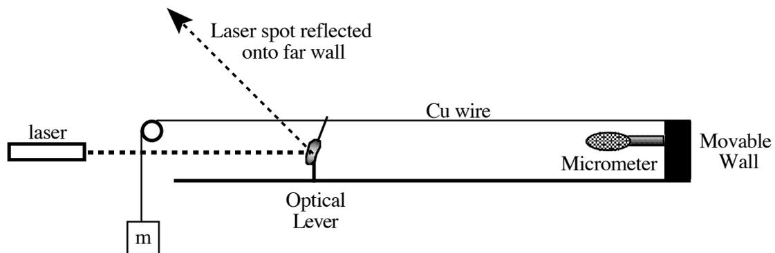
The micrometer is used to move the wire a known distance while observing the laser spot. This allows for a calibration of the laser spot position in terms of the actual deflection of the wire.
